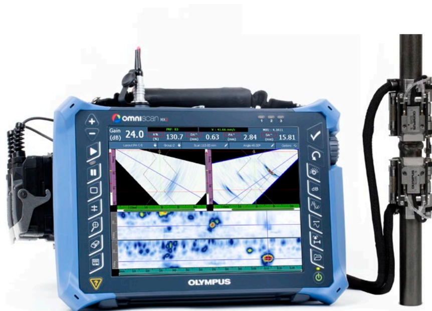
The COBRA scanner on a 0.84 in. pipe with two A15 PA probes with an OmniScan MX2 16:64 displaying two PA groups with sectorial scans and C-scans.
