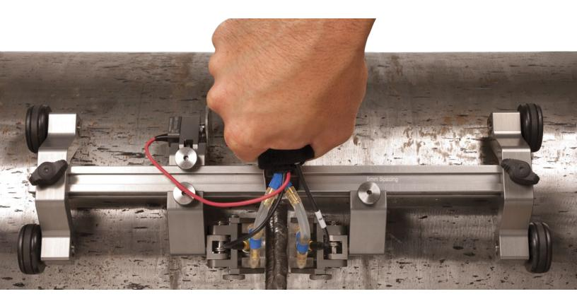
The new HST-Lite scanner is the perfect choice for costeffective, one-channel TOFD inspections when signal quality is important. The combination of magnetic wheels and springloaded probe holders offer the stability required to perform high quality, one-line inspections. The scanner can be operated using only one hand, and will attach to ferromagnetic surfaces even when in an upside-down position.
